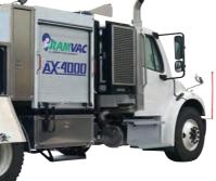
**Does It All**: This one machine provides the ability to pothole using a 4" port, as well as conduct major excavating utilizing a 6" port. The AX-4000 series offers standard payload capacities from 5,000 to 12,000 lbs. while its hydraulic rear door allows operators to dump spoils quickly and easily.
