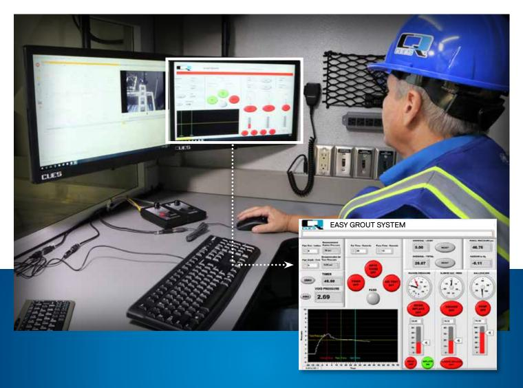
THE CUES EASY GROUT SYSTEM IS A COMPUTERIZED GROUT CONTROL SYSTEM DESIGNED TO CONSOLIDATE ALL VALVES, ELECTRICAL CONTROLS, ETC., INTO AN INSTRUMENTATION CABINET THAT CAN BE MOUNTED IN ANY LOCATION.
