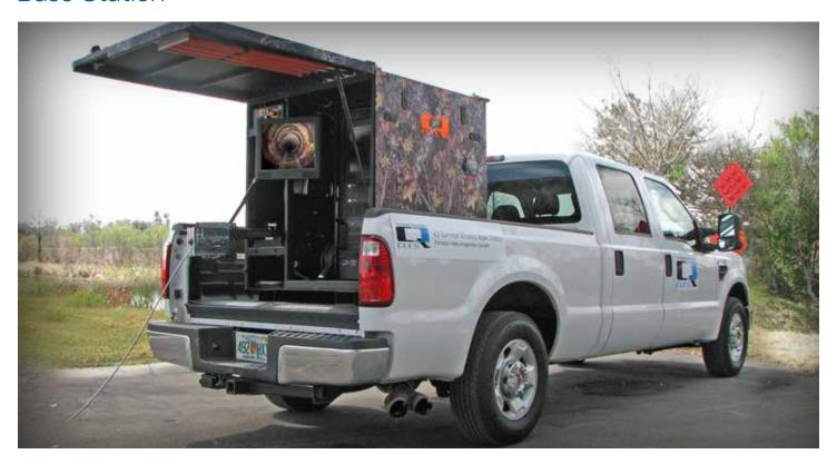
THE CUES K2 BASE STATION IS MOUNTED IN A COMPACT, RUGGED, WEATHER-PROOF ENCLOSURE AND CAN FIT INTO AN ATV, VAN, OR PICK-UP TRUCK TO ACCESS EASEMENTS AND HARD-TO-REACH AREAS.
