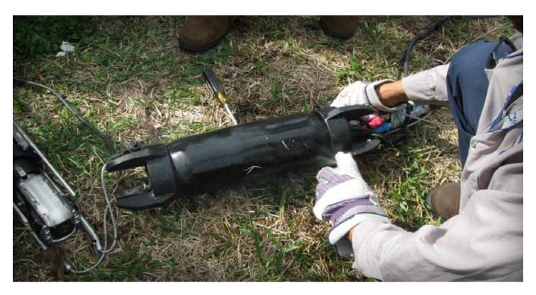
CUES LOW VOID PACKERS ARE LOW-VOLUME, CHEMICAL INJECTION, MULTI-GROUT PACKERS. LOW VOLUME PACKERS WORK WITH ACRYLAMIDES, URETHANE, AND OTHER COMMON CHEMICAL GROUTING MATERIALS.
