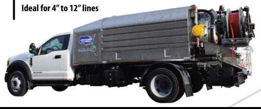
STAINLESS STEEL CONSTRUCTION: Debris tank, water tank, hose reel and full shroud
